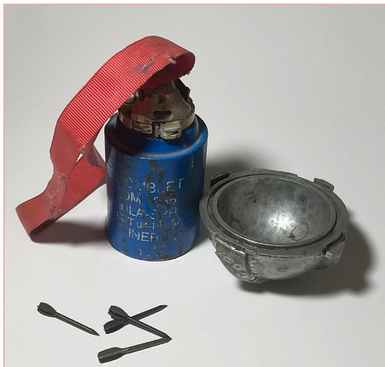
An inert M85 submunition, the remaining outer hemisphere of a BLU 26B (Guava) submunition, and four flechettes (photo R. Moyes).
