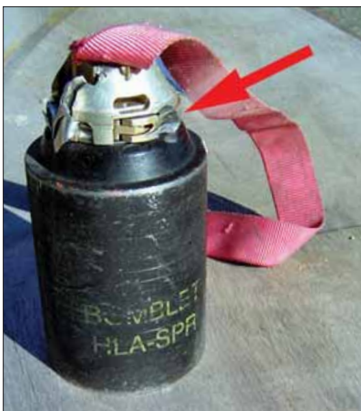
Figure 15: An example of a crimped fuze as a result of damage by an adjacent bomblet because of the levering effect during ejection. This dud is of the type DM1385 (another designation for M85) and was a result of test firings in Norway. Photo: Colin King
