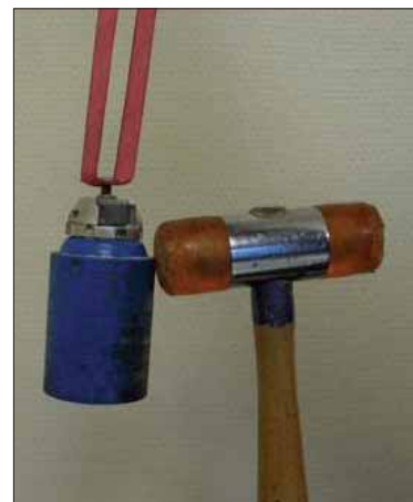
Figure 23: Tests with inert bomblets have shown that one hammer strike to the body of an M85 dud can be sufficient to make it arm. Photo: Ove Dullum/FFI.
