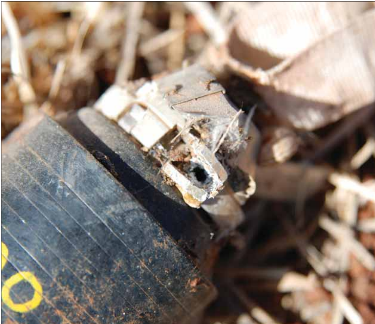
Figure 17: In some fuzes, the pyrotechnic SD delay had burned, but had not initiated the bomblet; this means that both the primary impact mechanism and the SD mechanism had failed. Photo: Amir Musanovic/NPA.
